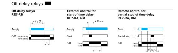
energised open closed t: adjustable Off-delay t = t1 + t2t: partial stop time
