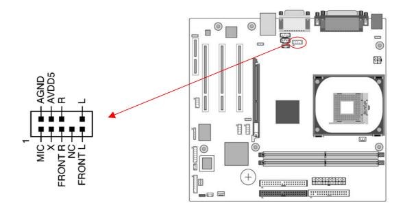
This connector gives you the option of a front-panel audio-jack cable ext. to be plugged into a special custom-designed system case.
