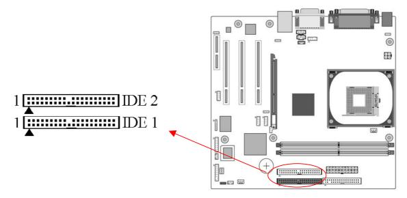
The motherboard has a 32-bit Enhanced PCI IDE and Ultra ATA66/100 controller that provides PIO mode 0~4, Bus Master, and Ultra ATA66/100 function. This connector is used for connecting 40 pin ATAPI devices.
