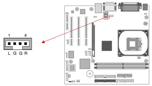
This connector is for the use of Auxiliary Audio-in Device.
