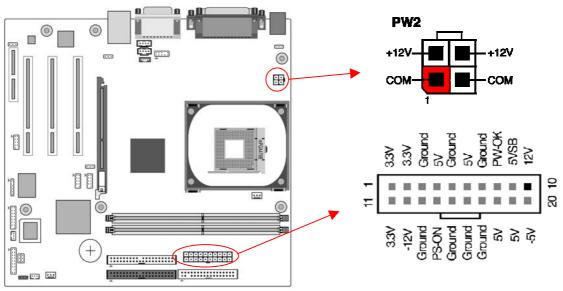
PW1 / 2 (ATX Power Supply Connector)
