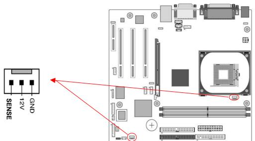
Connect the CPU/system/case-cooling fan to FAN1/2. The wiring and plugging may vary depending on the manufacturer. On standard fans, the yellow wire is positive (+12V), green is SENSE, and the black wire is ground.
