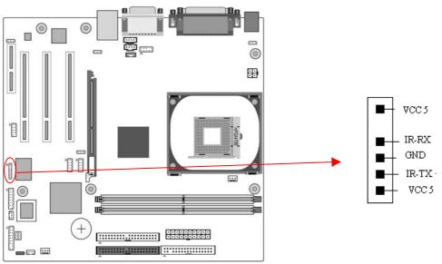
Select a COM2 Mode in BIOS's Integrated Peripherals menu the COM2 port to support IR function. (See section 3.4 Super I/O Device of Integrated Peripherals)
