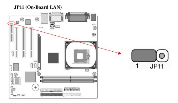
This function allows you to enable or disable the on-board LAN. You must set the jumper cap to pins 1-2 to enable or pins2-3 to disable this function.
