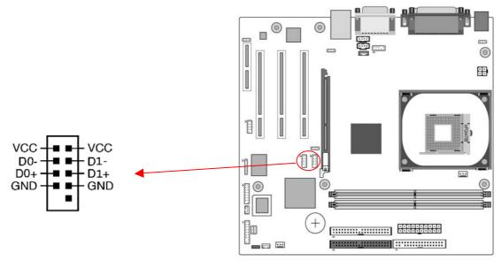
If you want to use an USB Keyboard, you must enable the USB keyboard support function in BIOS's Integrated Peripherals menu (See Section 3.4). This board contains an USB Host controller and a root hub with two connectors is included for an optional USB Adaptor (USB 2/3 and 4/5).
