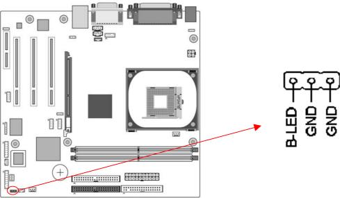
These features work entirely the same as the power indicator LED, both shows the system's power status. The only difference is that this one is blue while the other is red LED.
