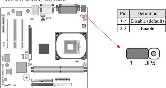
The PS/2 keyboard (hot key) can turn on the board. To use this function, select a hot key of your choice from BIOS's Power On Management screen ->Wake Up Events -> PS2 KB Wakeup option. You must also set this jumper's cap to pins 2-3 to use this function.
