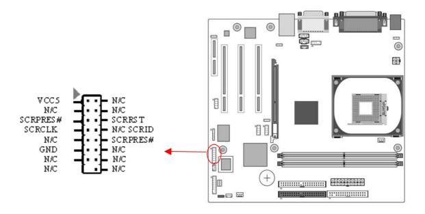
This connector must be connected to an optional Smart card reader.
