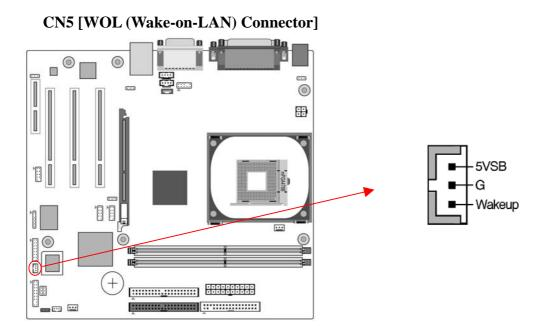
Enable the Wake Up On LAN selection in BIOS's Power Management Menu to use this function. The capability to remotely manage PCs on a network is a significant factor in reducing administrative and ownership costs. Magic Packet technology is designed to give WOL capability to LAN controller. This header is used to connect an add-in NIC (Network Interface Card) that gives WOL capability to the motherboard.
