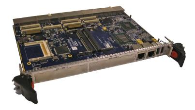
The CPB4912 is a PICMG 2.16-compliant packet switched backplane (PSB) processor blade based on the Intel® Core™ i7 processor. It combines high performance with low power, making it an ideal fit for telecommunications and Internet IP-based applications, as well as industrial control, testing services, and medical monitoring.
