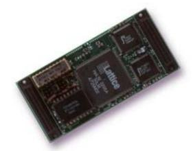
The Condor Engineering IP-708 module supports simultaneous receive and transmit of ARINC 708 data on a singlewide IP Module.
