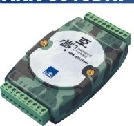
**Specifications and Features** Communication Interface Analog Output Interface Communication Method: RS-485 Channel: 1 channel heat-resistance differential input channel Interface: 2-line (Pt, Cu) Speed: 300bps~115.2Kbps 16-bit Resolution Communication Distance: 1200m/9600bps 10sps Sample Rate Analog Precision: ±0.05% Isolation Voltage: 3000VDC Power Supply Power Supply: 10V~30V Other Function Dual Watchdog Timer
