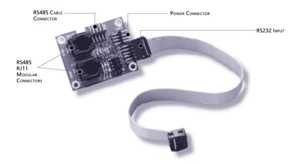
The RS485 Adapter offers a low cost, easy-to-use communications and networking interface that is ideally suited to a wide variety of embedded applications requiring low speed data transfer between two or more CPUs.
