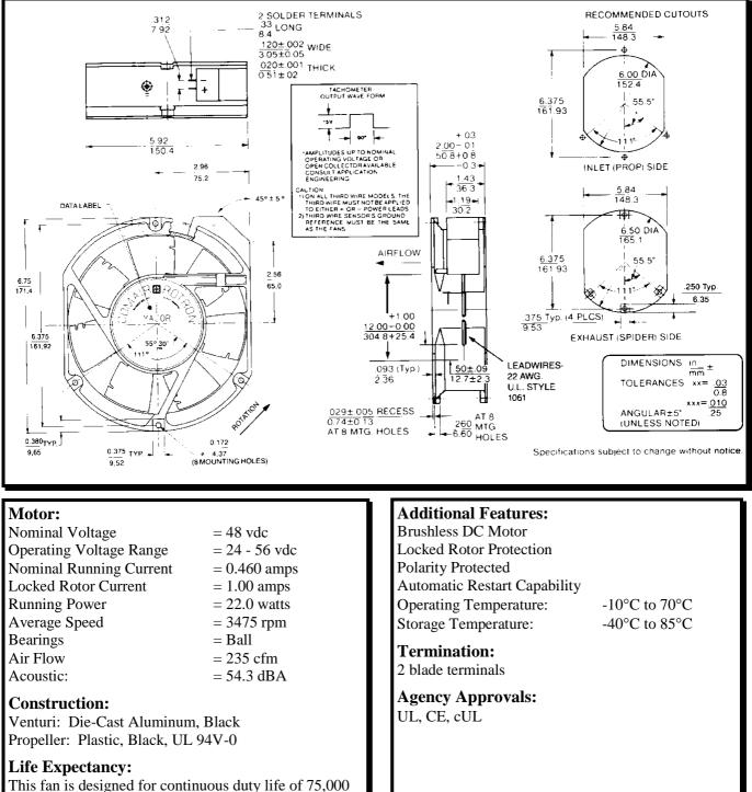
This fan is designed for continuous duty life of 75,000 hours at 40°C.
