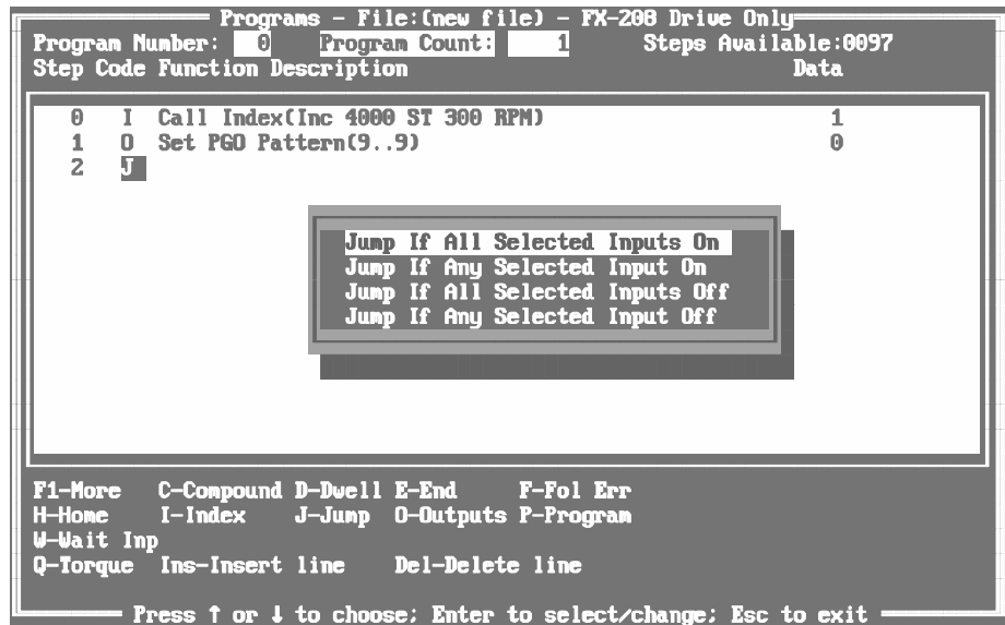
Figure 88 Jump on Input Pattern Commands Window
