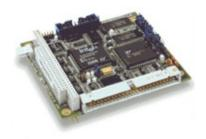
Datalight's ROM-DOS is a low-cost 'workalike' of MS-DOS 6.22, with extra features for the embedded environment. The PC/104 format is an industrial form factor measuring 3.8" x 3.5" (96mm x 90mm).
