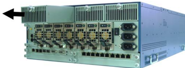
Figure 41 : Hot-Swapping Cooling Fan Trays
