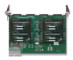
The CEI-600 is a flexible, space-saving. ARINC and multi-protocol solution for CompactPCI bus computers. Based on rugged and versatile modular technology (also known as IndustryPack), the CEI-600 provides the proven advantage of open system design while supplying a large number of low cost ARINC 429, ARINC 573, ARINC 708, MIL-STD-1553 and other interfaces on a single board.
