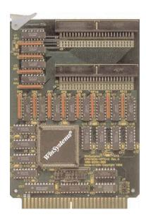
**Opto Isolation** - Each input line is optically isolated from others and from the bus interface circuits. The isolation voltage rating between the input and output of the photocoupler device exceeds 1500V.
