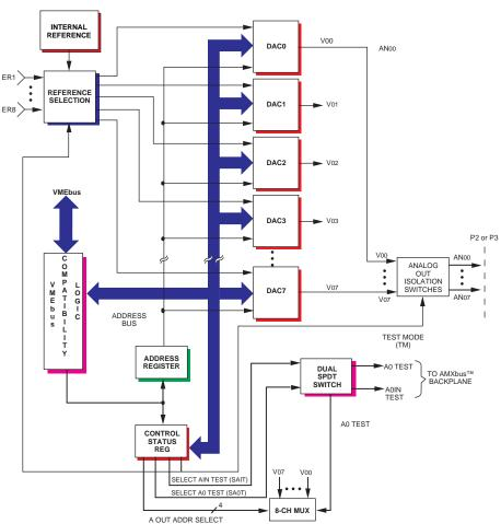
Figure 1. VMIVME-4105 8-Channel Multiplying Analog Output Board
