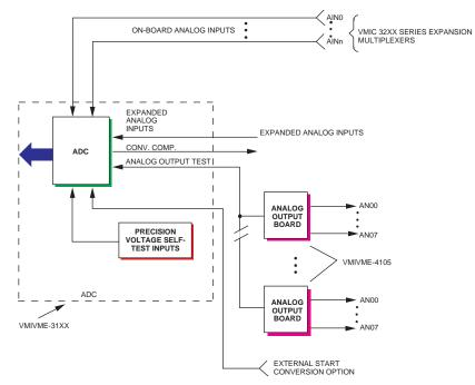
Figure 2. Simplified Functional Multiplying DAC Subsystem Configuration with Built-in-Test
