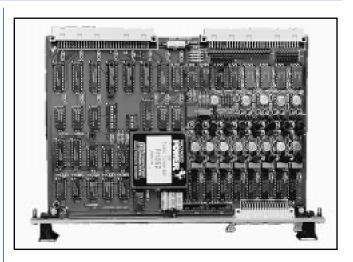
**Analog Output Testing:** Any one of the eight analog outputs may be switched to the analog output test bus (Test Bus 2). This bus is routed through the P2 AMXbus analog backplane to an Analog-to-Digital Converter (ADC) board which is used to verify each DAC channel on the VMIVME-4105 board.
