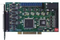
8-channel isolated 16-bit D/A output; 32-channel TTL digital input, 16-channel TTL digital output; continuous analog signal output
