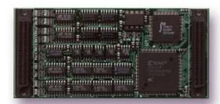
Condor Engineering has developed a powerful and versatile way to provide interfaces to ARINC 573 Harvard Bi-Phase and BPRZ (Bi-Polar Return to Zero) databuses. This unique solution is built on the rugged, crossarchitecture IP Module platform (also known as IndustryPack). IP Modules are standards-based I/O mezzanine cards (about the size of a business card), that mount onto host carrier boards (PC/AT, VME, VXI, PCI, CompactPCI, etc.), enabling crossplatform portability.
