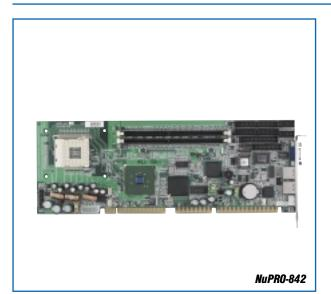
••• The NuPRO-842's Pentium 4 processor, Dual Gigabit Ethernet ports provide the highest performance computing solution available today. As a 32 bit, 33Mhz PCI Single Board Computer, the NuPRO-842 supports PICMG 1.0 Backplane for computing servers, telecommunication computers, and Industrial Controller.
