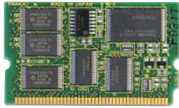
CNC built-in flash memory Max. 8MB
