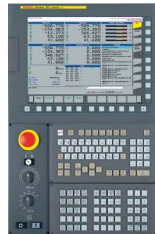
15-inch color LCD unit, QWERTY keyboard, standard machine operator's panel
