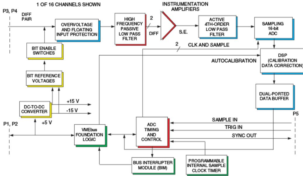
Figure 1. VMIVME-3123 Functional Block Diagram
