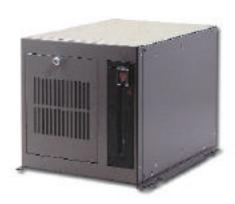
IRC-306S is a compact and rugged 6-slot node chassis for industrial controller in the space limited application. Since CD-ROM is the most common device for installing s/w, it is equipped with a notebook PC CD-ROM drive for easy installation of the necessary OS or application s/w. Its rugged, sturdy, full-sealed and well-cooled steel chassis is designed to withstand heavy shock, dust, humidity, vibration and high temperature in the harsh environments.
