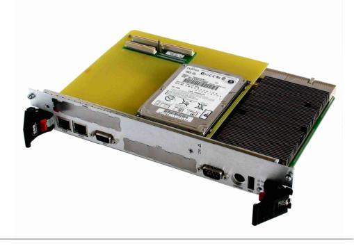
**CP9** is a 6U CompactPCI all-in-one CPU board with a low power Intel<sup>®</sup> Pentium<sup>®</sup> M processor and dual Gigabit Ethernet channels. The CP9 supports full hot swap and is capable of being used in a system or non-system (peripheral) slot. Adhering to the PICMG 2.16 dual Ethernet specification, the CP9 supports the 64-bit/66 MHz CompactPCI bus.
