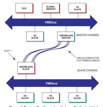
Figure 2. Typical Configuration Using a Dedicated Link
