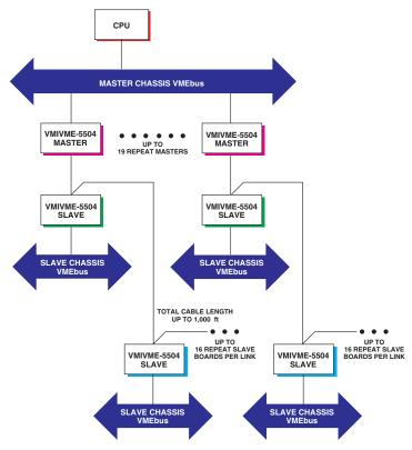
**Figure 1. Typical Multidrop Configuration**
