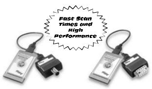
The SST DeviceNet Pro PC Card (PCMCIA) connects your PC Card bus computer to DeviceNet. The Pro card is a high-performance version of the SST DeviceNet PC Card and is compatible with all applications written for the SST DeviceNet PC Card.
