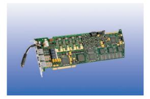
The full-size, single PCI slot assembly can function as a standalone solution or can be combined with other hardware via a CT Bus interface (H.100). The DI/0408-LS is a second-generation board that reduces the overall hardware to a single baseboard from the previous baseboard and daughterboard design, while increasing resource availability and options. It is designed to comply with a range of international approvals.
