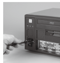
Plug ring-lock securely fastens the power cord
