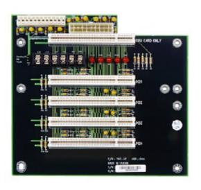
1 PCI System Bus; 4 PCI expansion Bus Slots
