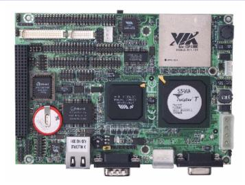
VIA C3<sup>™</sup>, series Processor SubCompact Board with LCD, LVDS, TV-out, TV-out, Ethernet, Audio, CompactFlash<sup>™</sup>, USB & 4
