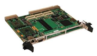
Diversified Technology's CPB4612 PICMG 2.16-compliant packet switched backplane (PSB) processor blade combines high performance with low power for telecom and Internet IP-based applications.
