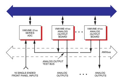
The AMXbus backplane may be replaced with a standard P2 VME expansion bus and user-supplied jumper wires on the user I/O pins. The VMIC AMXbus backplane is available in printed circuit form in 5, 9, or 19 slots. The AMXbus backplane is designed to provide enhanced noise immunity and is recommended for most applications.
