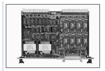
**VMEbus Access:** Address modifier bits are jumper-selectable to support nonprivileged short I/O or supervisory short I/O access. The board is factory configured for supervisory short I/O access.
