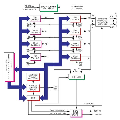
Figure 1. VMIVME-4116 Board Functional Block Diagram
