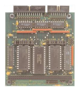
Read operation for event-counting applications. Special logic is included so that the contents of each counter can be read "on the fly" without having to inhibit the clock input.
