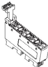
Hook the RTB end into the mounting base end and rotate until it locks into place.
