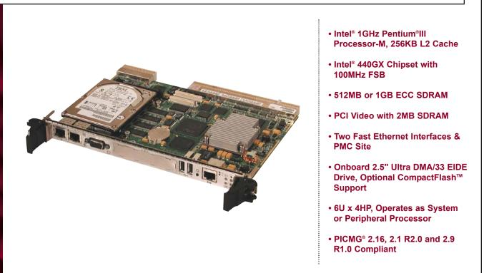
Diversified Technology's modular cPB-4321 hot-swap CompactPCI<sup>™</sup> processor blade, compliant with the PICMG 2.16 packet switched backplane (PSB) open standard, offers superb value with a feature set optimized for Internet, telecom and industrial control applications.
