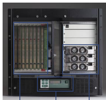
8-slot backplane with H.110 CT Bus LCM for system status (MIC-3921) 560 W ATX 2+1 redundant power supply
