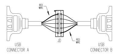
Figure 9. USB 1.1 Connector Orientation Diagram
