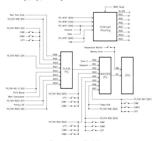
Figure 10. Interrupt Circuit Diagram
