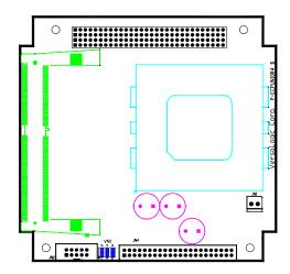
Figure 6. Jumper Block Locations (CPU Module)
