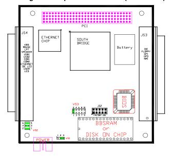
Figure 7. Jumper Block Locations (I/O Module)
