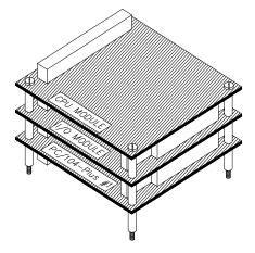
Figure 3. PC/104-Plus Card Added to Bottom of Stack
