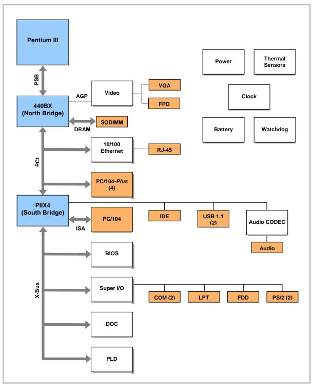
Figure 1. EPM-CPU-10 Block Diagram
