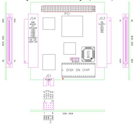
Figure 5. Connector Location Diagram (I/O Module)
