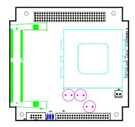
Figure 4. Connector Location Diagram (CPU Module)
