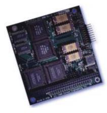
The CEI-400 has been designed to conform to industry standard PC/104 specifications, is based on proven Condor technology, and facilitates simplified access to ARINC 429 databus functionality. Available in multiple configurations, the CEI-400 will support a maximum of 8 ARINC 429 or ARINC 575 channels per module.
