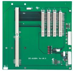
Max. Systems: 1 System Slots: 1 x EPI Expansion Slots: 4 x PCI Power: ATX/AT Order Information: EPI-6105P4
