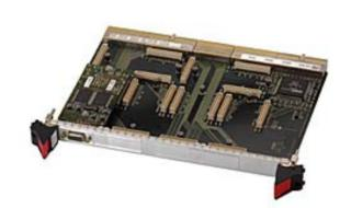
The D202 is a 6U PC-MIP carrier board for universal I/O on the CompactPCI bus or on the PXI bus. You can install up to six PC-MIPs on the D202, with four Type I/II and two Type I PC-MIPs.
