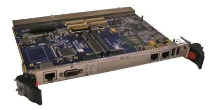
DTI's CPB4912V is a PICMG 2.16-compliant packet switched backplane (PSB) CompactPCI blade based on the Intel® Core™ i7 processor. The board provides a single piece solution by combining storage, video and networking all on one 6U blade. By utilizing high performance processing with low power, the CPB4912V is an ideal fit for video intensive applications in telecom, industrial control, medical/image monitoring and testing services.
