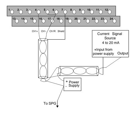
Figure 11-5 Current Input Connections (4 to 20 mA)
