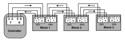
**NOTE:** CC represents the communication connections at the top of the block modules.
