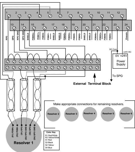
**Block Input Resolver Module Screw Terminals**
