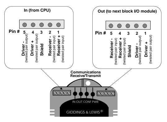
Figure 7-8 Pinouts for Communication Connectors
