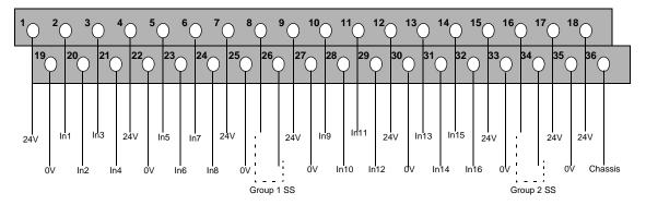
Figure 4-2 Screw Terminal Connector Assignments
