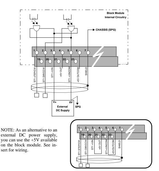
Figure 10-3 Connections for One Stepper Output
