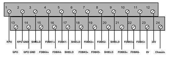
Figure 9-2 Connections for the Block Input Resolver Terminals
