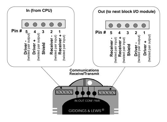
Figure 13-3 Pinouts for Communication Connectors
