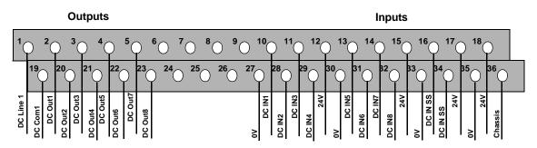
Figure 5-2 Screw Terminal Connection Assignments
