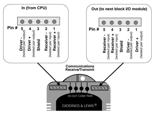
Figure 6-3. Pinouts for Communication Connectors
