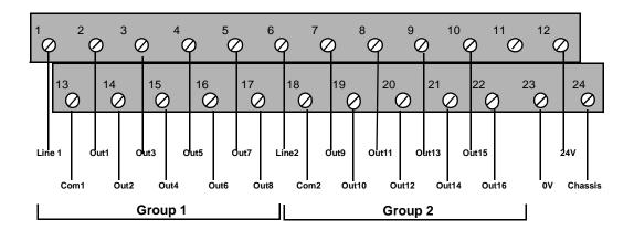
Figure 3-2 Screw Terminal Connection Assignments
