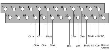
Figure 12-2 Screw Terminal Connector Assignments
