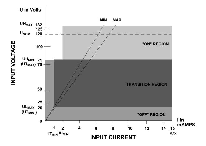
Figure 8-5 Input Characteristics Compared to IEC Standards
