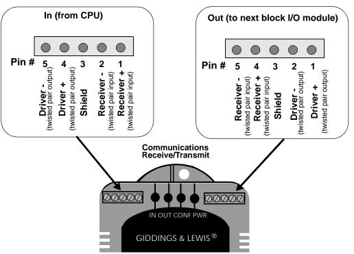
Figure 3-4 Pinouts for Communication Connectors
