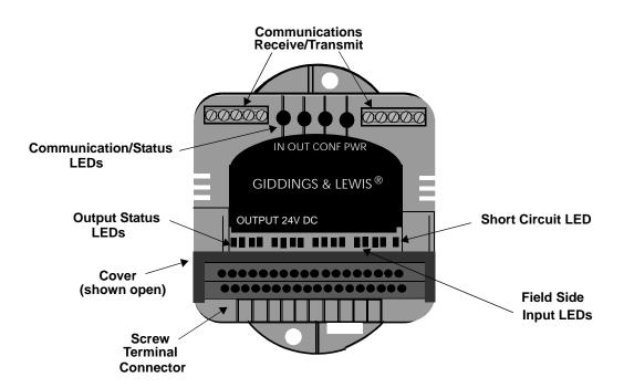
Figure 15-1 Block 24V DC 8In/8 Out Module/J
