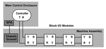
The distance between Block I/O can be up to 200 feet
