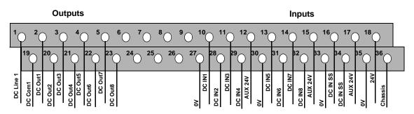
Figure 15-2 Screw Terminal Connection Assignments
