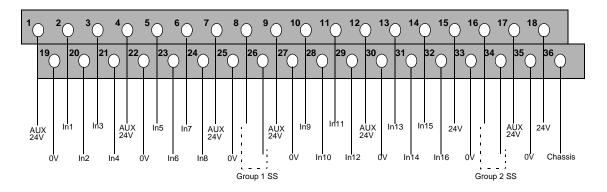
Figure 14-2 Screw Terminal Connector Assignments
