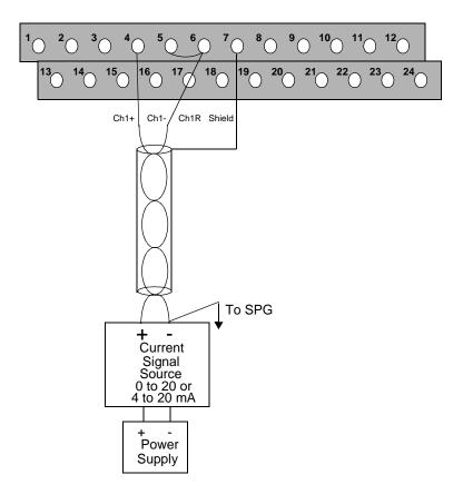
An alternative method of connecting a two wire 4 to 20 mA current device is shown in Figure 11-5. Place a jumper between the - input and the  $250\Omega$  resistor input.
