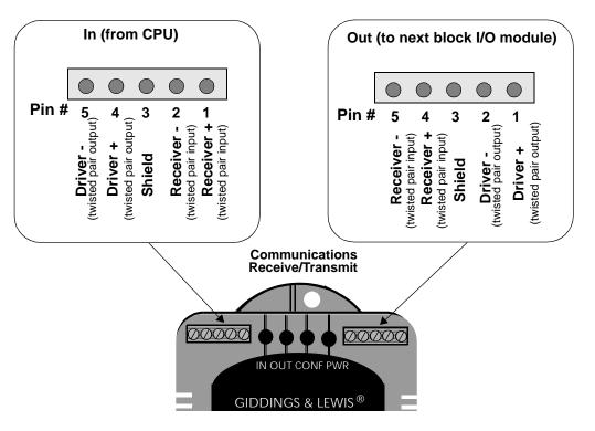
Figure 9-5 Pinouts for Communication Connectors
