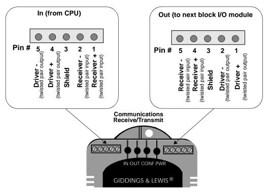
Figure 12-4 Pinouts for Communication Connectors
