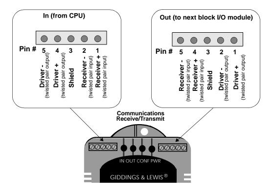
Figure 8-4 Pinouts for Communication Connectors
