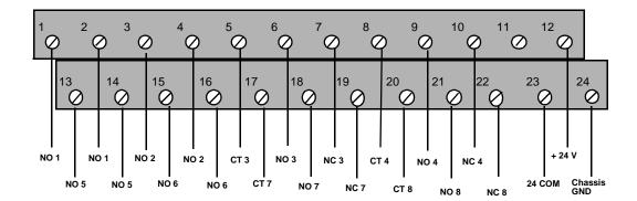
Figure 7-2 Screw Terminal Connector Assignments
