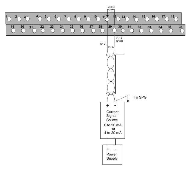
NOTE: The accuracy of the currrent input can be no more accurate than the accuracy of the 250  $\Omega$  resistor used.
