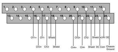
Figure 13-2 Screw Terminal Connector Assignments
