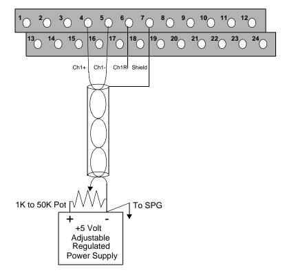
Figure 11-6 Adding an External Potentiometer
