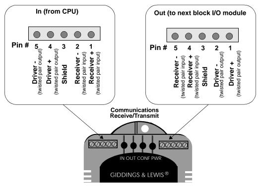
Figure 11-7 Pinouts for Communication Connectors
