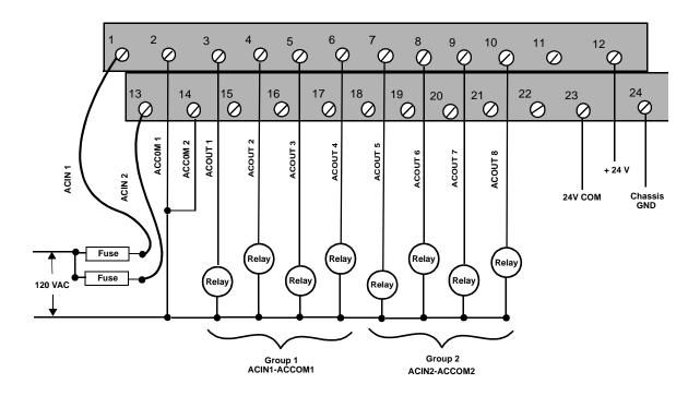
Figure 6-2. Screw Terminal Connections
