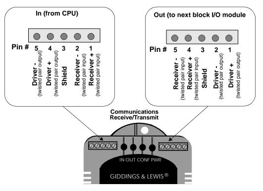
Figure 16-8 Pinouts for Communication Connectors
