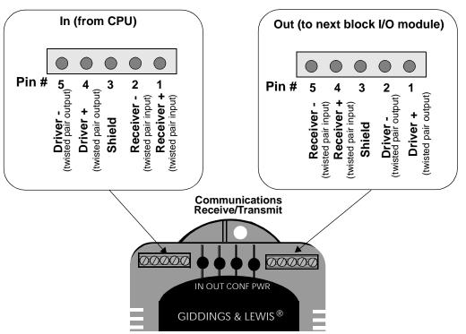
Figure 4-4 Pinouts for Communication Connectors
