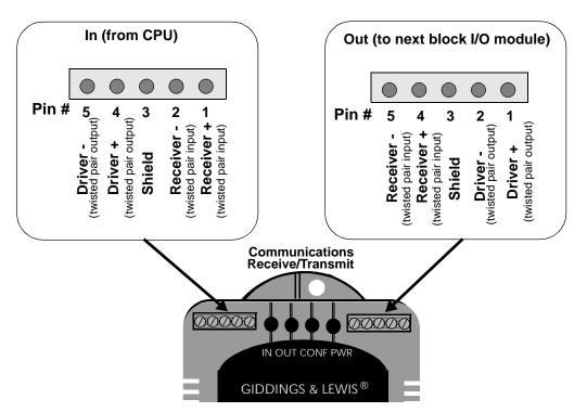
Figure 10-10 Pinouts for Communication Connectors
