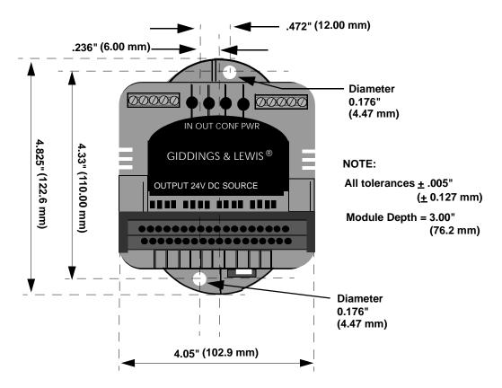
Figure 2-2 Mounting Dimensions
