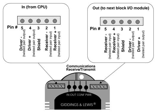
Figure 14-4 Pinouts for Communication Connectors
