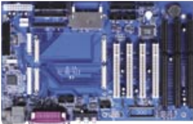
ETX-DB-7SR-R20 Full Function ETX Baseboard with LCD/CRT VGA, Audio, DOC, CF II & D I/O
