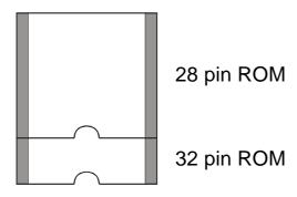
32 pin ROMs should take up the entire socket and should be fitted in the orientation shown in the 'Default Link Position' diagram.
