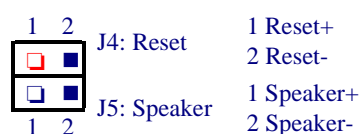
Figure 3-6 J4 Reset Header & J5 Speaker Header
