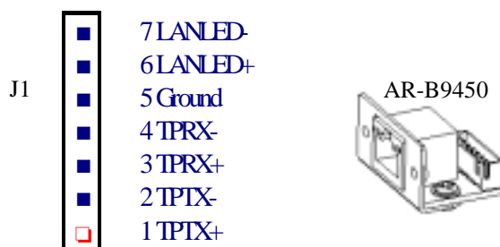
Figure 3-3 Ethernet Connector Pin Assignments and AR-B9450 Ethernet Adapter Module
