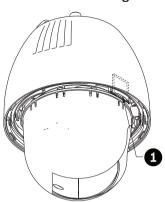
AUTODOME 7000 - Slot for SD card
