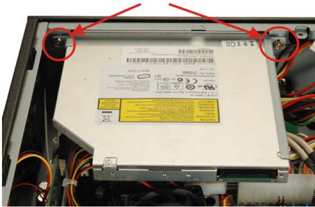
Figure 11: Fasten Optical Drive Screws
