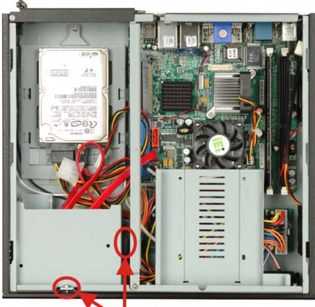
Figure 12: Hard Drive Bracket Screws
