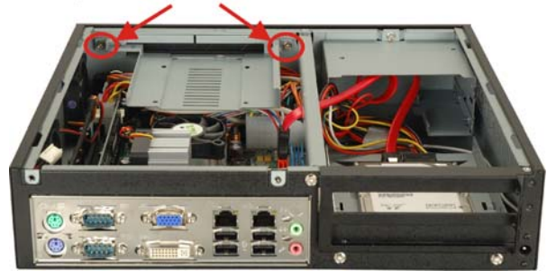
Figure 4: Optical Drive Bracket Screws
