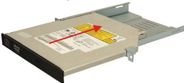
Figure 7: Slide the Optical Drive
