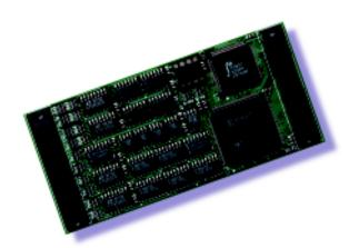
The Condor IP-CSDB is an intelligent IP Module (IndustryPack-compatible) interface for the Commercial Standard Digital Bus avionics protocol and RS-422 applications. Up to 4 pairs of fully independent CSDB channels are supported. Standard features include on-board buffering, internal wrap, timetagging, along with programmable selection of bus speeds parity and gap time.
