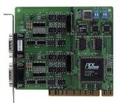
Industio CP-132 Series 2 Port RS-422/485 Industrial Communication Board for PCI 2 RS-422/485 ports
