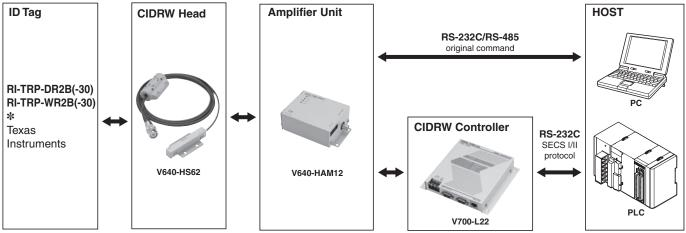
Note: 1. Use of the V700-L11 ID Link Unit enables the Amplifier Unit to be removed/installed while the CIDRW System remains turned ON in the event of a malfunction or during maintenance.
