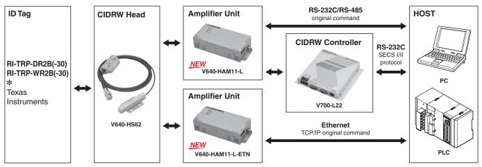
Note: 1. Use of the V700-L11 ID Link Unit enables the Amplifier Unit to be removed/installed while the CIDRW System remains turned ON in the event of a malfunction or during maintenance.
