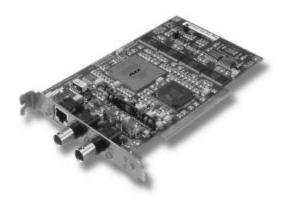
The SST ControlNet PCI card connects your PCI bus computer to ControlNet.
