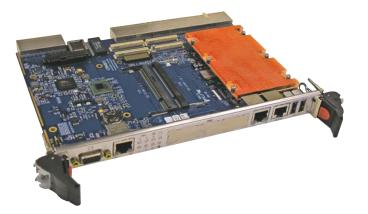
Diversified Technology's CPB4811 PICMG<sup>®</sup> 2.16-compliant packet switched backplane (PSB) processor blade combines high performance with low power for telecom and Internet IP-based applications.
