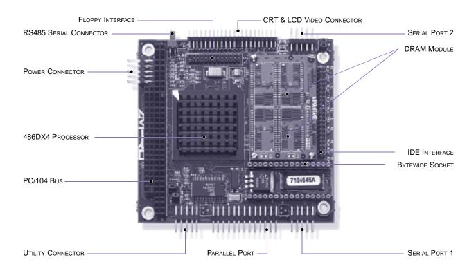
The CoreModule/4GV, along with the CoreModule/4GE, is the first of Ampro's new family of high integration PC/104 CPUs. These modules pack 486 processing power together with all standard embedded PC product features—including CPU and memory subsystems, communications ports and disk interfaces—plus key additional features into less than 14 square inches of board space. This high level of integration allows a single module to serve a wide range of embedded applications.
