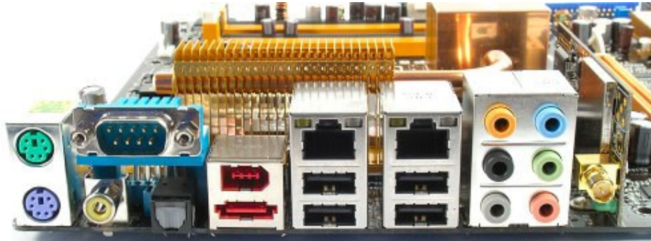
Top down, left to right - PS/2, COM port, coaxial and optical S/PDIF, FireWire-400, eSATA, Gigabit LAN RJ45, USB 2.0, 8-channel analog audio and WiFi antenna connector.
